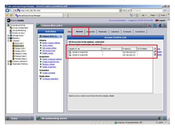
Figure 1: ACL Entries for the EqualLogic Volumes
